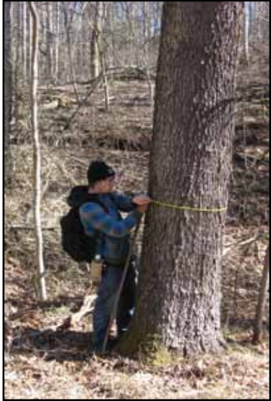
"Diameter at Breast Height" (DBH) refers to the measurement of tree diameter at a height of 4.5 ft above the ground. DBH provides a standard place to measure diameter which is important because trees are often tapered.
