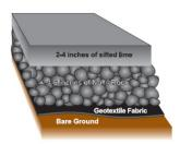
Heavy use areas are constructed by placing geotextile fabric under crushed stone and dense grade aggregate. These areas provide a dry place for feeding or loafing during wet weather or when pasture is limited.
