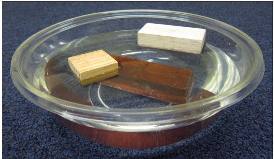
**Figure 1-3.** The densities of different wood species can vary considerably. Here we see balsa (density = 0.1 g/cm<sup>3</sup>) floating very high in the water; southern pine (density = 0.55 g/cm<sup>3</sup>) floating but with about half of its volume submerged; and cocobolo, a tropical species (density = 1.1 g/cm<sup>3</sup>), completely submerged. The density of water is 62.4 lb/ft<sup>3</sup>, or 1.0 g/cm<sup>3</sup>.
