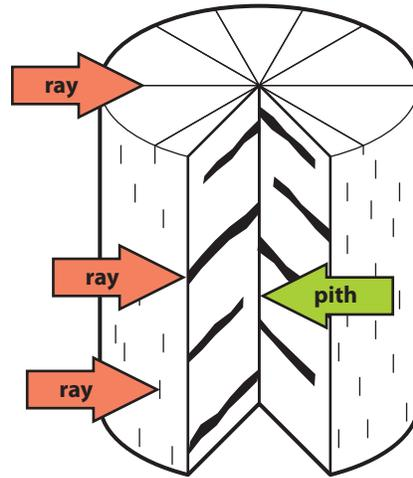
**Figure 1-1.** This sketch shows how rays extend from the cambial layer just beneath the bark (where ray cross-sections appear as short thin lines) toward the pith in the center of the tree. Rays may appear to be discontinuous because the plane of the cut and the plane of the rays may be slightly different, especially if the grain has small local deviations. Note the pith that runs longitudinally in the center of the tree parallel to the fibers.
