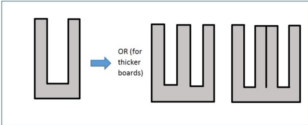
**Figure 27.** A single pair of prongs is appropriate for 4/4 boards, but thicker boards are usually cut somewhat differently. You are looking at representations of the end grain in these diagrams. For 4/4 boards, the prongs should be about one-quarter of the board thickness.
