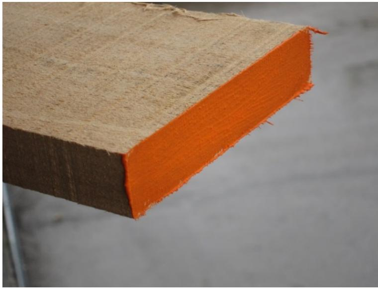
The front illustration shows a sample board coated with B.O.S.S.<sup>®</sup> (Bright Orange Sample Sealer), made by U-C Coatings Corporation.
