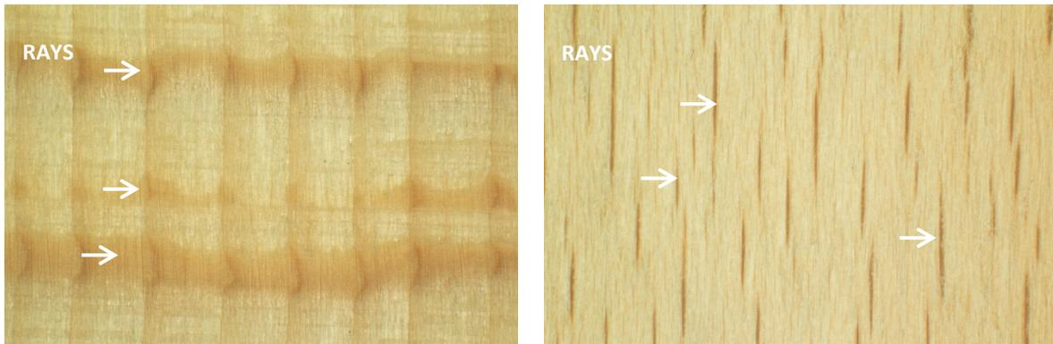
**Figure 15.** American beech: Some rays are labelled on the radial (quartersawn) and tangential (flatsawn) faces, respectively. The quartersawn face exposes the side of the rays, making them look like ribbons; what you see on a flatsawn board is the ray ends. Each ray is made up of many individual ray cells, as shown in Figure 10 below.
