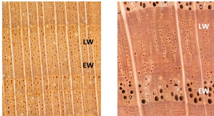
**Figure 8.** These micrographs are of the end grain of two different wood species. A diffuse porous species (hard maple) is on the left, and a ring porous species (red oak) is on the right. EW and LW stand for earlywood and latewood, respectively. Earlywood and latewood together make up one year's growth (a growth ring).
