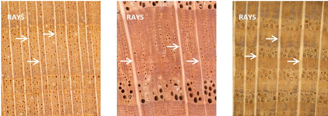
**Figure 10.** A few of the rays are labelled on the end grain for each of these micrographs (of hard maple, red oak and white oak, shown above from left to right). The rays in the oaks are significantly wider than those in maple. These broad rays help to distinguish the oaks from other species.
