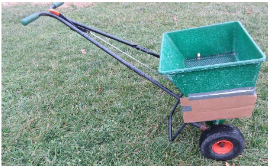
Figure 3. Lawn fertilizer spreader with cardboard taped to one side to keep fertilizer off of impervious surfaces such as a driveway, street or sidewalk.
