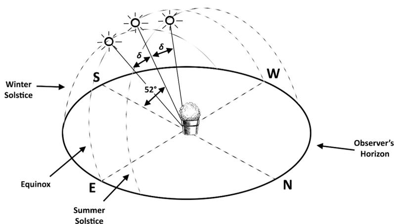
**Figure 2.** The direction and intensity of direct solar radiation striking a container sidewall varies throughout the day and time of year. (Lexington latitude =  $38^\circ$ ; solar angle during equinox =  $52^\circ$ ; tilt angle ( $\delta$ ) =  $23.5^\circ$ ). Illustration by Joshua Knight
