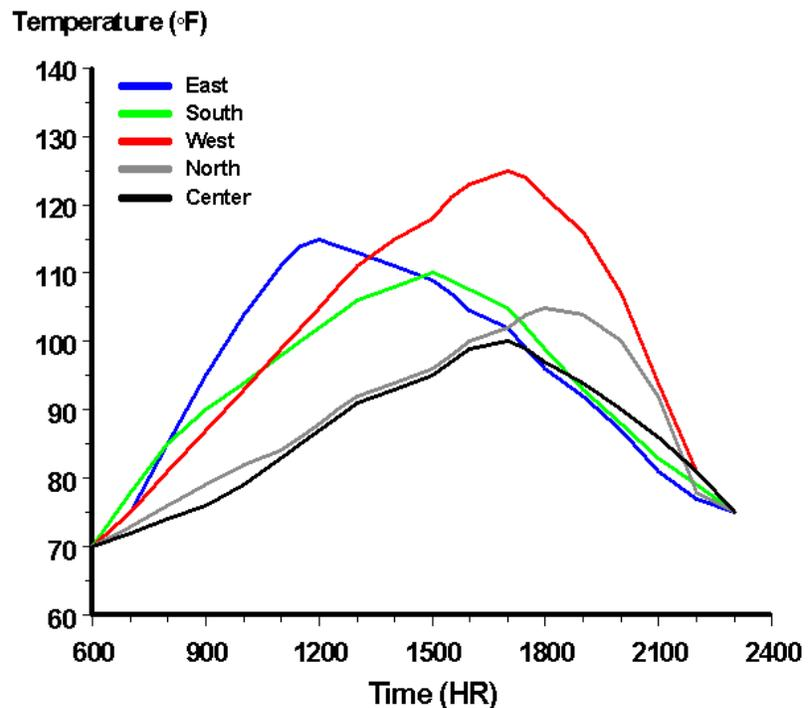
**Figure 1.** Root-zone temperature fluctuations 1 inch from the sidewall in the east, south, west, and north quadrants and in the center of the substrate in a #2 container throughout a mid-summer day in Lexington, Kentucky
