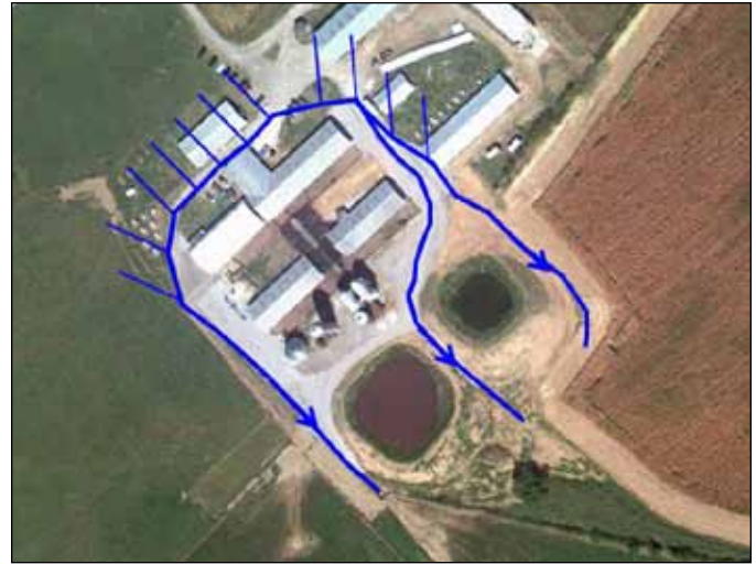
Figure 4. Installing clean water diversions increased capacity in the liquid storage ponds.
