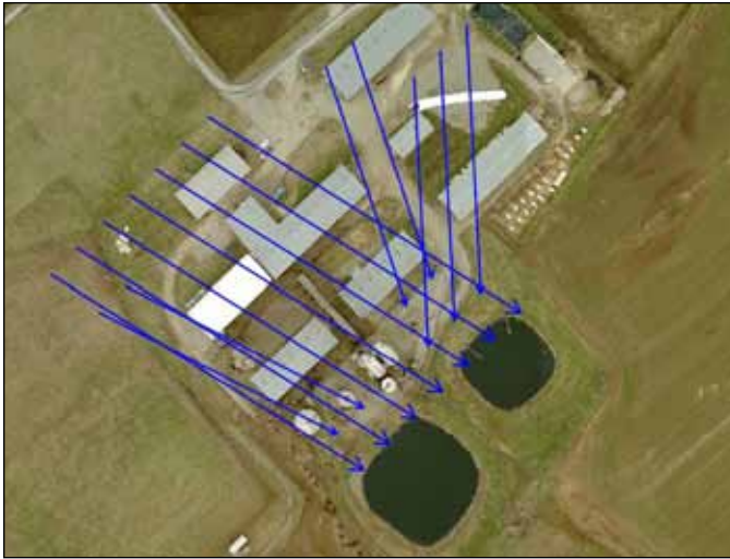
Figure 3. Before clean water diversion methods were implemented, the production area drained into the liquid storage ponds.
