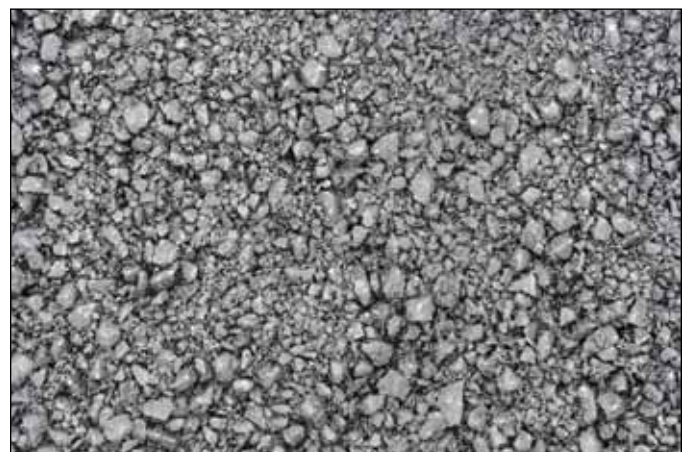
Figure 5. Porous asphalt is very similar in appearance to conventional asphalt except it has a rougher texture.
