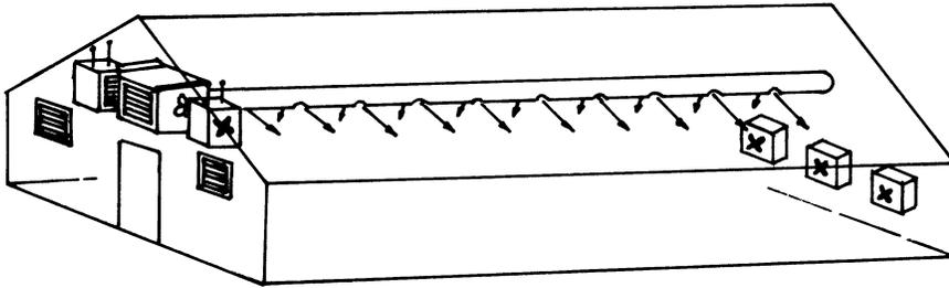
b. Unit heaters and a special poly-tube fan housing
