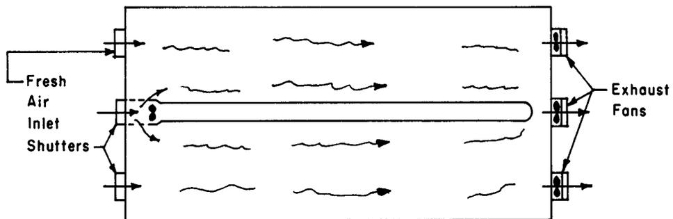
Figure 5: Total summer ventilation is provided by additional high-volume exhaust fans, thus rendering the poly-tube less effective for summer use.
