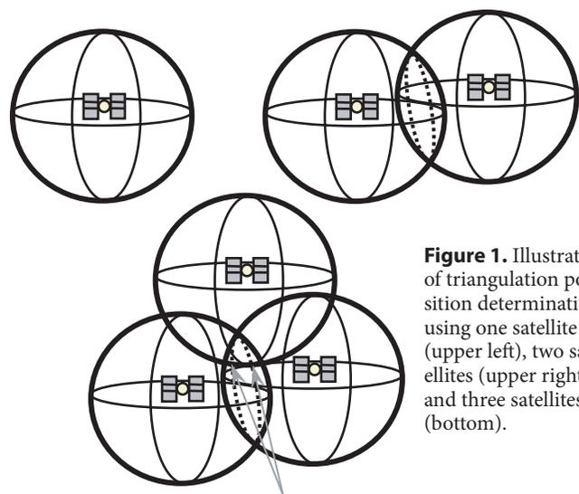
**Figure 1.** Illustration of triangulation position determination using one satellite (upper left), two satellites (upper right), and three satellites (bottom).
