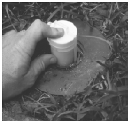
c. Inspection of monitoring device (note presence of termites).
