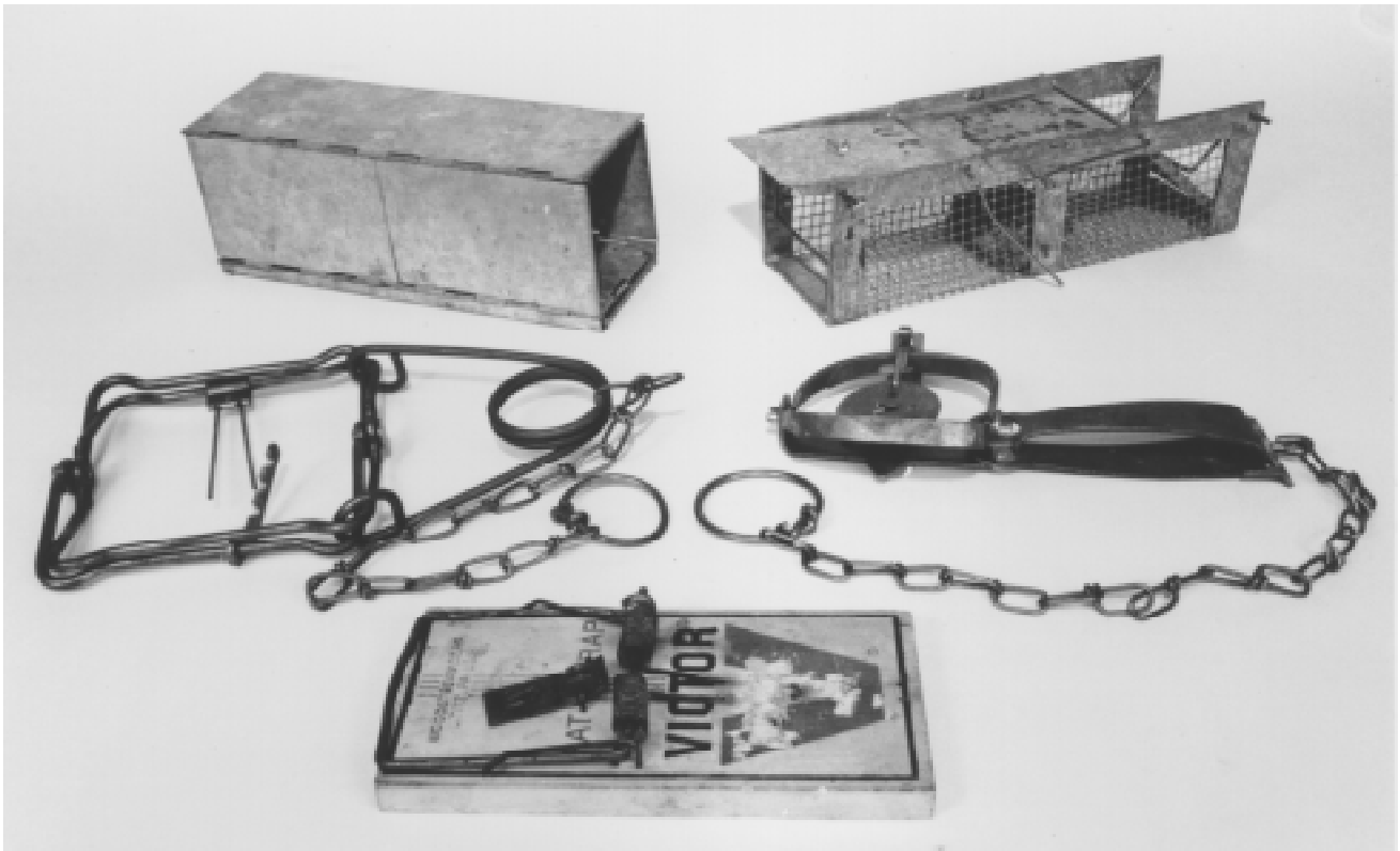
Figure 2. Clockwise from the bottom: a rat snap-trap, a body-grip trap (in set position), a Sherman live-trap, a cage trap (in set position), and a leg-hold trap.
