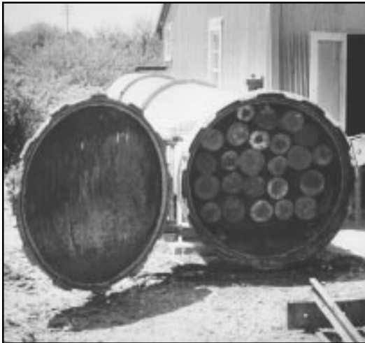
figure 2 - Wood is pressure treated in a large cylinder.
