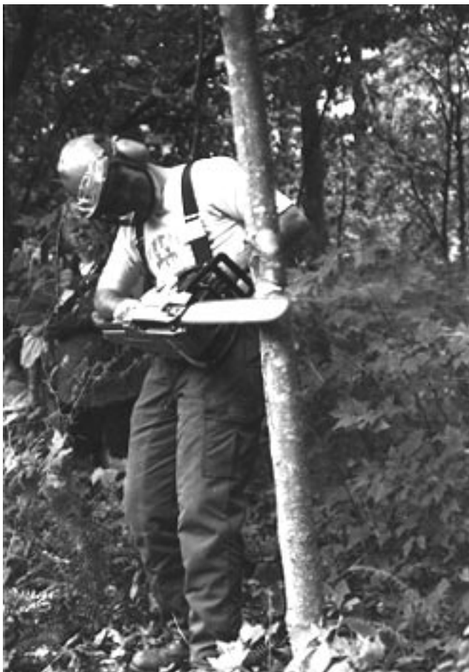
Figure 2. A Tennessee Valley Authority harvesting specialist demonstrates how the open face hinge should operate.
