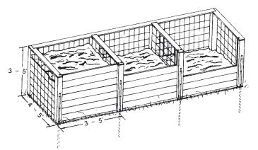
Figure 3. Bin composter with three chambers.
