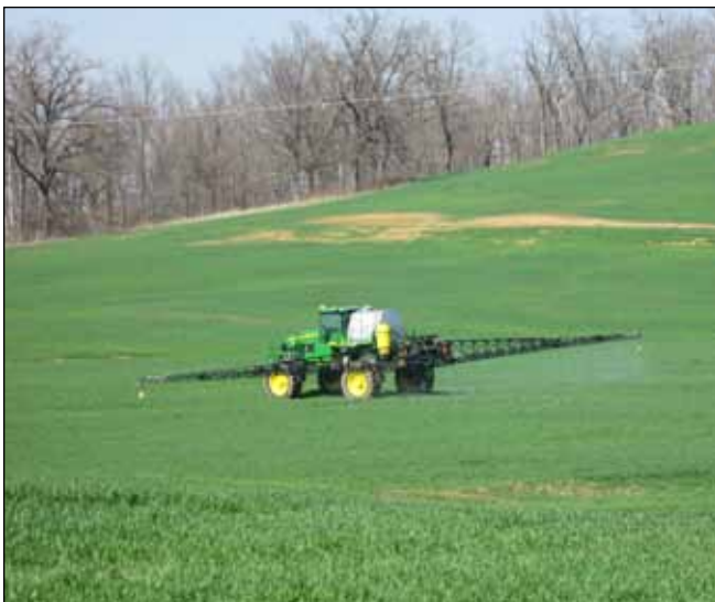
Photo 5-7. Most nitrogen fertilizer is applied as a liquid urea ammonium nitrate (UAN) and 28 or 32% N. By using stream bars or stream jet style nozzles, leaf burn from the UAN is minimized. Granular nitrogen (usually urea) can also be applied.
