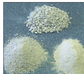
Figure 4. An ag lime sample divided into the three sizes: coarser than 10-mesh (top), 10 to 50-mesh (lower left), and finer than 50-mesh (lower right).
