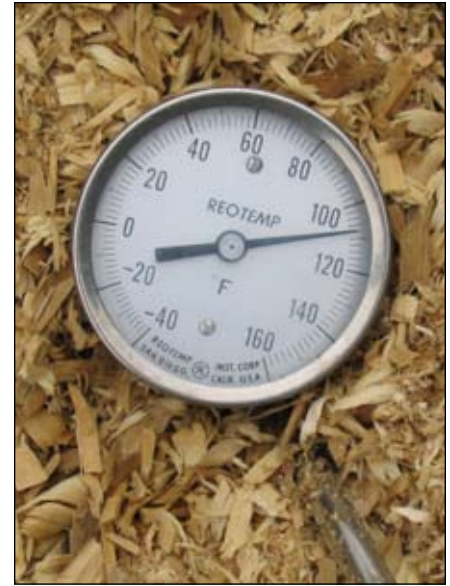
Figure 2. An example of a dial type thermometer. (This pile needs to warm up.)
