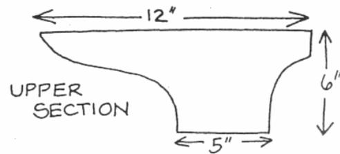
Sand until smooth; join with glue and screws from the bottom.
