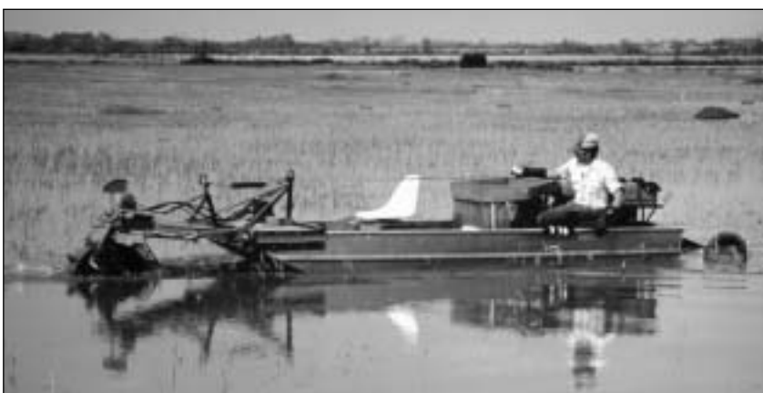
Figure 7. A crawfish harvesting boat powered by a forward-mounted hydraulic wheel (photo, LSU AgCenter).
