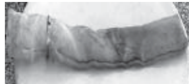
Figure 9. Filter socks can be made from plastic window screen and stitched with monofilament fishing line. Shoe shops do an excellent job inexpensively.
