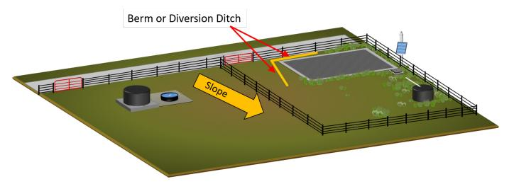
Figure 4. A rain trap with an upland diversion created to redirect flows that may contain pollutants. (Illustration by Donnie Stamper)
