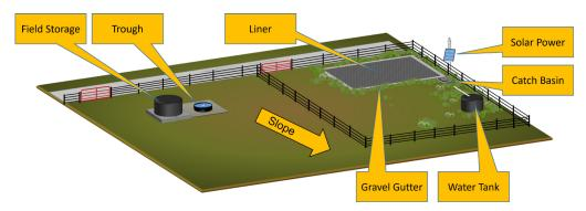
Figure 3. A solar-powered rain trap. (Illustration by Donnie Stamper)
