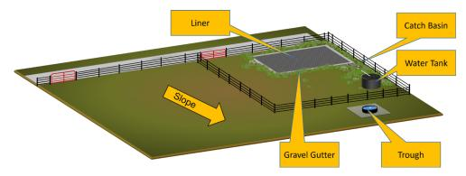
Figure 2. A gravity-fed rain trap. A fence excludes livestock from the trap. (Illustration by Donnie Stamper)
