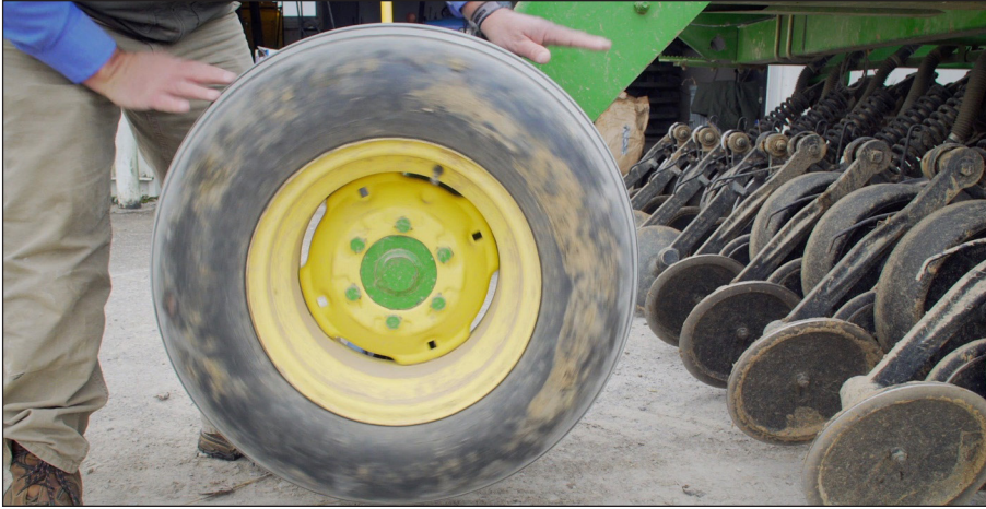
Figure 3. Determine the circumference of the drive wheel by direct measurement or by using the following formula: circumference in feet = 3.14 x diameter of drive wheel in feet.
